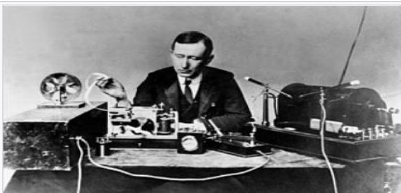
Guglielmo Marconi who built the first radio receivers, with his early spark transmitter ( right ) and coherer receiver ( left ) from the 1890s. The receiver records the Morse code on paper tape
